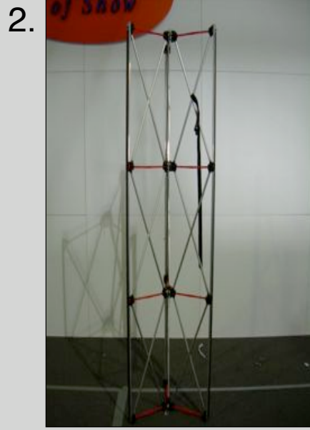
2. Take the tower out of the case and pop it out. The hub with the yellow goes on the bottom and the the hub with black faces the top.
