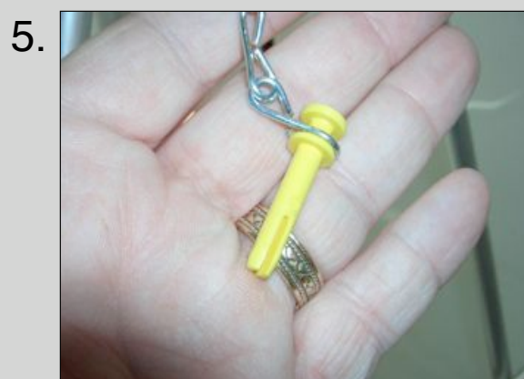
5. Each tower comes with a yellow pin (4) and that is attached to the hub with a Jack chain. This pin will go through the opening of the that the hubs have.
