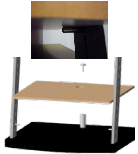
Place the pins into the groove of the octanorm. Also place the standoff barrels into the base of the kiosk. Slide the bottom of the counter until it the counter base rest on the pins that are on the octanorm. (See picture above for pins detail).
