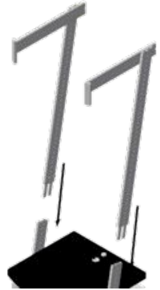
Place the top section of the octanorm into the bottom section of the octanorm. Use hardware that is provided.
